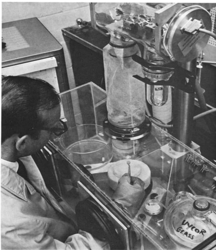
Fig. 4. Sample placement in electrobalance at controlled humidity.
